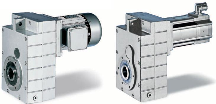
Our axial shaft-mounted helical gearboxes are short, and capable of transmitting high torque levels. The low level of backlash offered by the toothing ensures the highest precision. Optimised tooth profiles and ground gears ensure both low-noise operation and low backlash.
